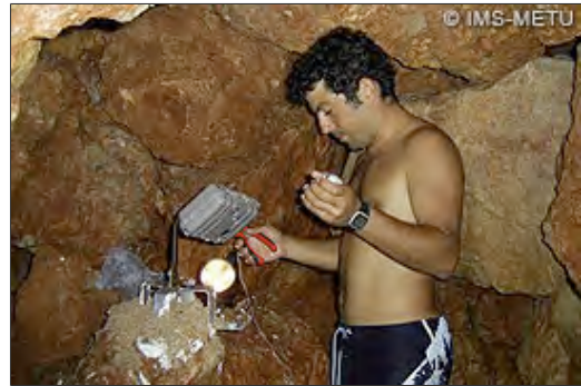
Installing a photo-trap in a cave on the Cilician coast.
